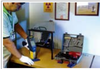
Handheld XRF for RoHS Compliance Testing
